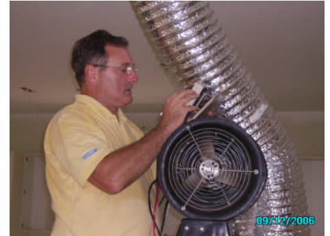
EBS Auditor performs duct leakage test
